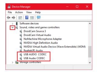
Note that I now have two (yes, two!) that look almost the same. From the previous figure, I know that the **USB Audio CODEC** is the **FT-991A**. The next new device (**USB AUDIO CODEC**, all uppercase) is my **SignaLink**. I'm making note of that as I continue. I will only be working with the **USB Audio CODEC** on the FT-991A for the remainder of this article.
