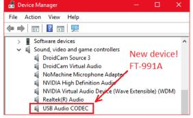
**USB Audio CODEC** is my FT-991A. I also use a SignaLink connected to another transceiver. Let's see what happens when I plug it in without disconnecting the FT-991A.
