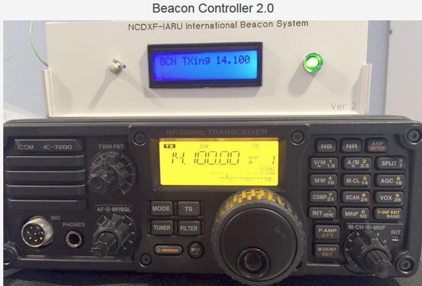
ICOM IC-7200 and custom controller using Arduino platform
