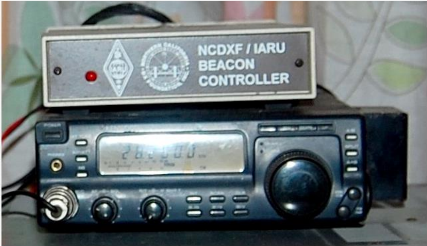
Kenwood – TS-50 and custom controller using 8748 microcontroller
